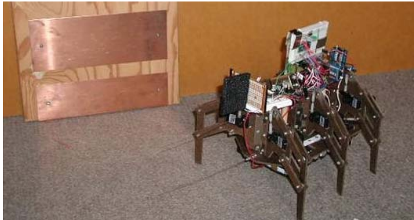
Figure 2: ServoBot with charging station (power supplied by a power supply). The ServoBot charges its capacitors through probes (can be seen on the front of the robot) that are aligned to make contact with charging plates.
