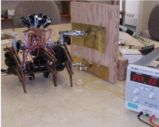
Figure 2a. The ServoBot equipped with capacitors and probes during charging.
