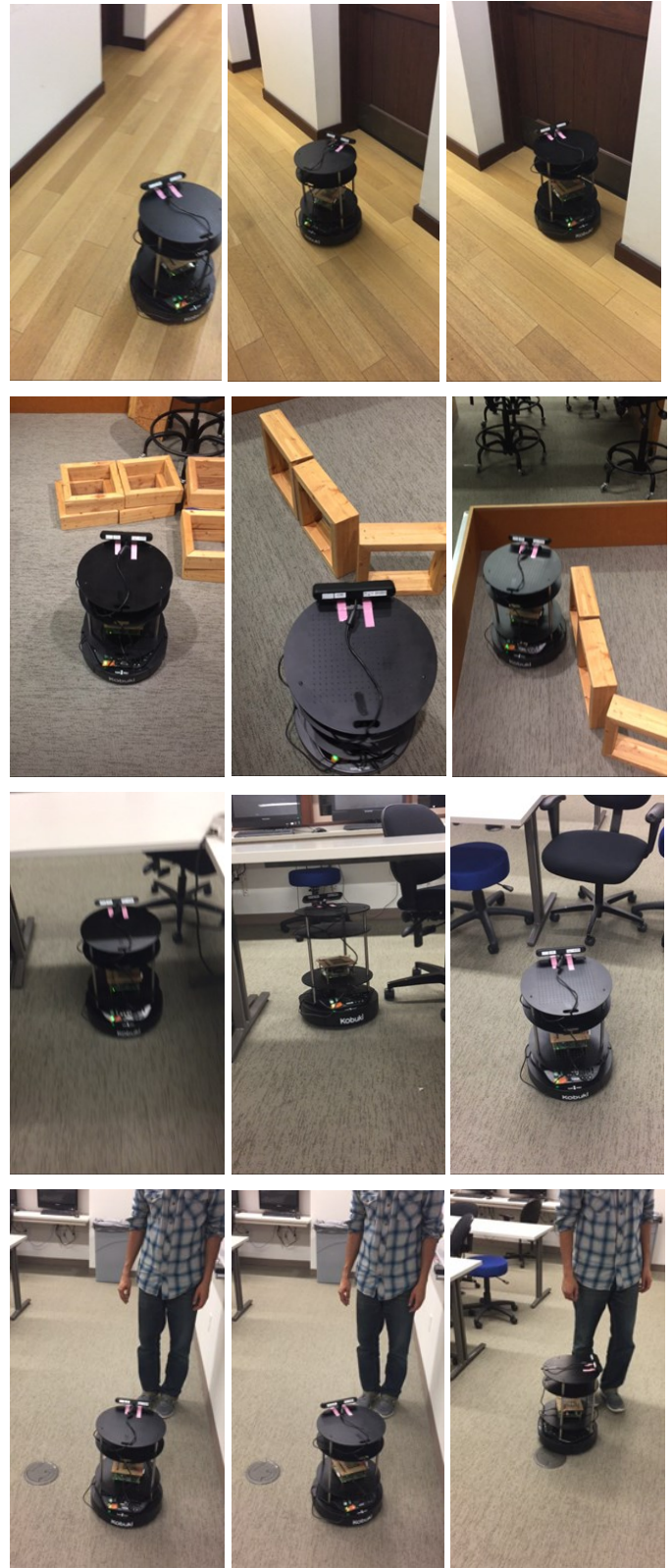
Fig. 4. New environments not seen by the robot during training: first row: hall; second row: colony space; third row: other lab with lower chairs/tables; fourth row: person.
