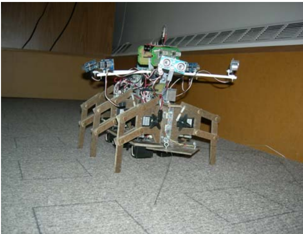
Figure 2. Photo of the prey with 6 range finding SONAR sensors and two antennas (wire touch sensors)
