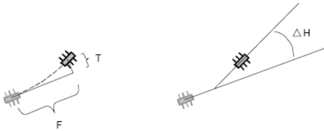
Fig 3. Gait Cycle Turn Measurements. The left diagram shows F and T. F is the distance moved forward (relative to the start position heading). T is the distance moved in the turn direction (perpendicular to the start position heading). The right diagram shows \Delta H , which is the change in heading from before to after turn execution.
