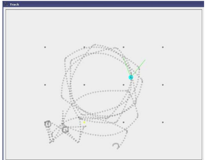
Fig. 8. Path of robot using best chromosome found by EE with one chromosome per robot after 20000 steps.
