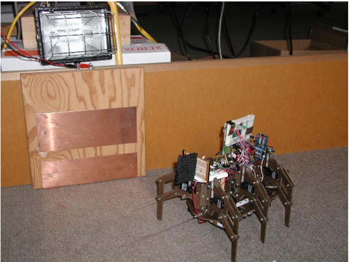
Figure 1. The robot, power station with its metal plates, and light source.
