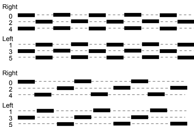
Figure 6: Rough terrain gaits. The dark areas are times when the leg's foot is off the ground. The top diagram shows a sample tripod gait produced using the high stepping leg cycles. This gait lacked the support needed to keep the heavy robot off the ground at all times. The bottom diagram shows a sample gait produced after anytime learning with fitness biasing was applied to gait generation. The second gait seldom had more than two legs off the ground at one time, so it provided the support needed to hold the robot off the ground. This gait is very similar to the slow metachronal wave used by some slow walking insects.
