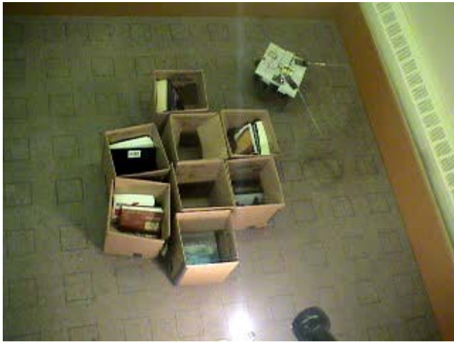
Fig. 1. Photograph of the colony space. The hexapod robot appears as a white square since mostly what one can see is the sensor base. Two tactile sensors are also clearly seen coming from the sensor base. The obstacles are 30cm x 30cm boxes; shown in the Central Mountain configuration. The light is a normal incandescent light since only one light sensor was used in each of the learned sensor morphology.
