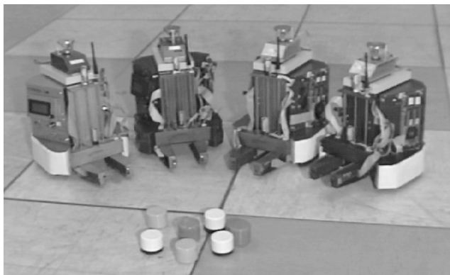
Figure 6: The family of four IS Robotics mobile robots used in the group behavior experiments. The robots are equipped with IRs, contact sensors, grippers, position sensors, and radio communication.
