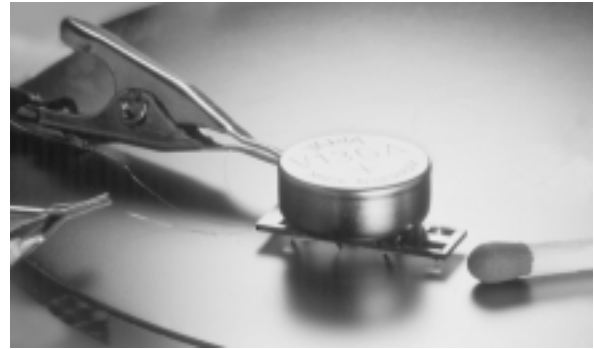
Fig. 5. The micro-robot during a load test. The load of 2500 mg is equivalent to maximum 625 mg/leg (or more than 30 times the weight of robot itself). The power supply is maintained through three 30 \mu\text{m} thin and 5 to 10 cm long bonding wires of gold.
